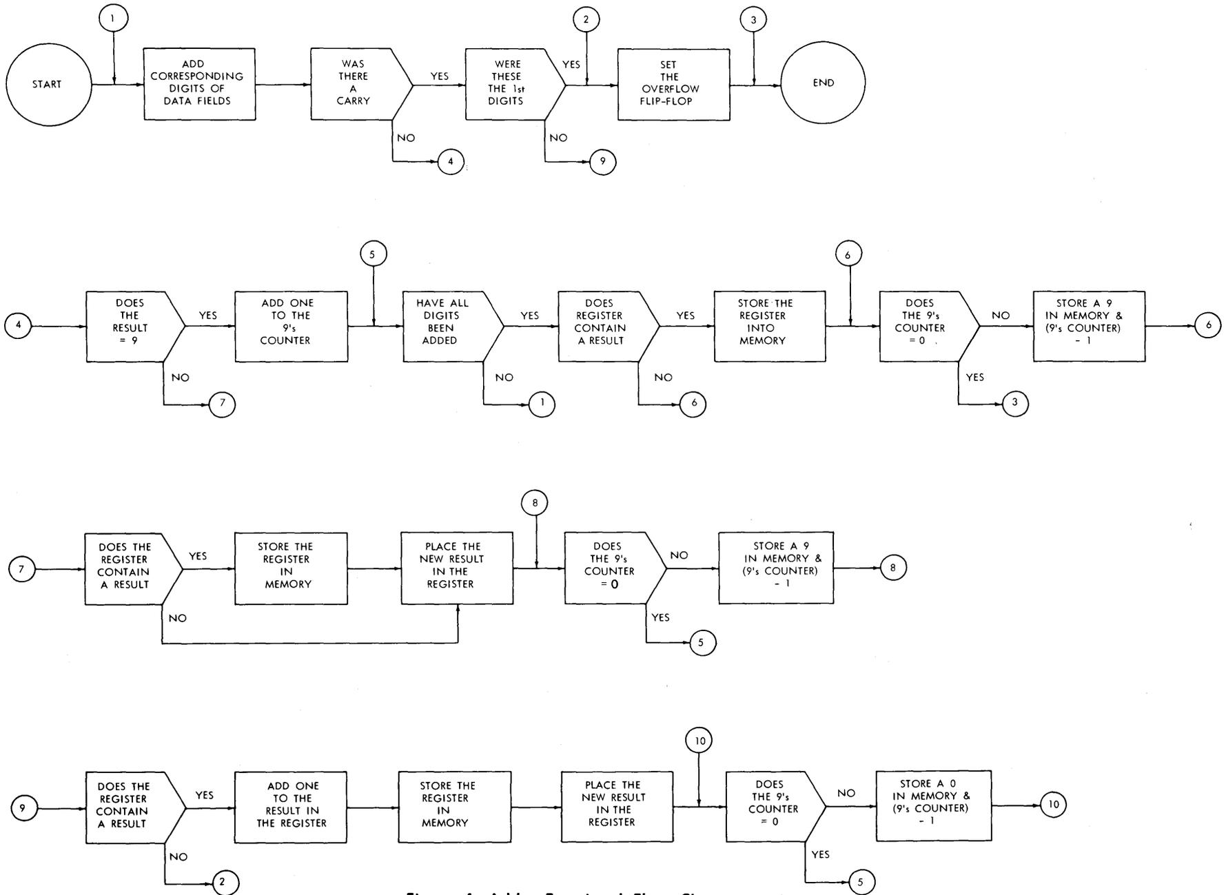
Figure 4. Adder Functional Flow Chart
