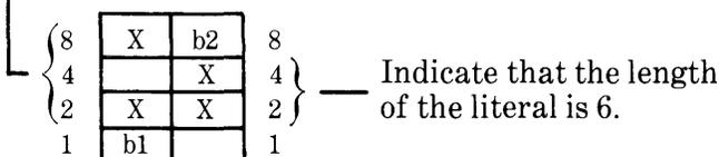
In the example, b1 and b2 both being OFF indicate an unsigned numeric representation. The A syllable contains a literal of six unsigned numeric digits.
