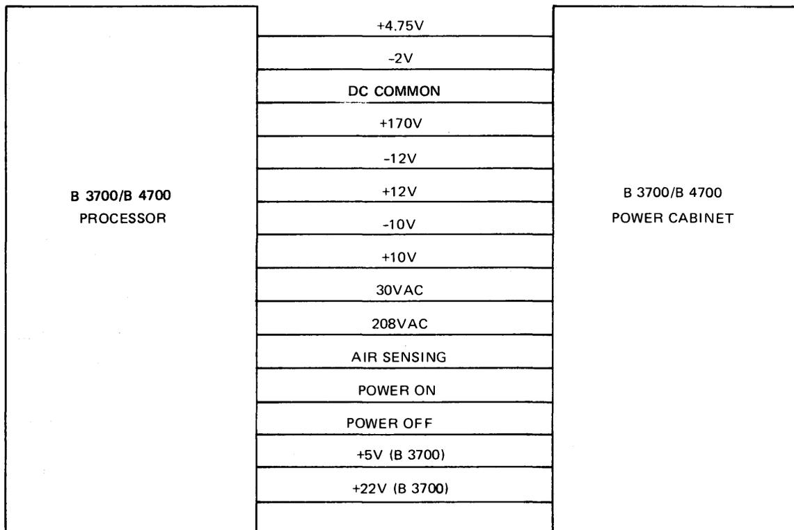
Figure 14. Processor Voltages
