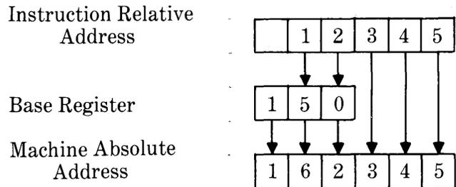
Assume further that the program has indicated that an instruction is to be indexed by the contents of index register 1. The final absolute location would be derived as shown below:
